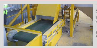
The Can Sorter is specifically designed for the separation of non-ferrous beverage cans from dry recyclable materials. The Can Sorter ECS is a low-cost alternative to larger Eddy Current unit, for applications that do not require high specification machines.
