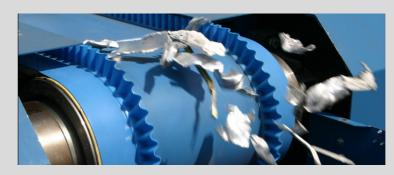
For applications that require separation of finer non-ferrous particles, Eccentric ECS units can be supplied. The Eccentric rotor differs in that the magnet system is of a smaller diameter and is located in an eccentric position to the outer rotor drum. The magnet system is positioned close to the surface, giving maximum repulsion where the conveyed materials discharge from the rotor.
