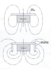
If the operating gap is 300mm or higher, the Type K incorporates a Tri-polar design as standard. The tri-polar design utilizes massive steel side members to effectively give three poles across the bottom face of the magnet, intensifying the field in the centre of the magnet block. Master Magnets also recommend a tri Polar design for operating heights below 300mm, where there is need to separate small ferrous contaminates such as nails and screws.
