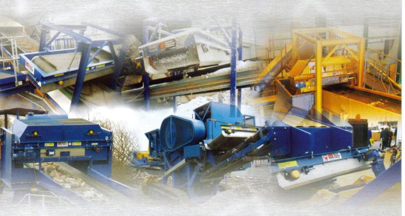
Master Magnets range of permanent and electro overband magnets is one of the widest available. They are used for the continual and safe removal of tramp metal from conveyor lines, vibratory feeders and chutes.
