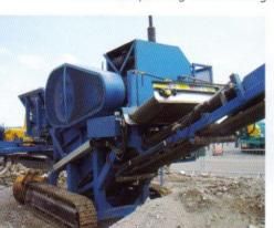
The Type K self cleaning magnet is mainly used in the quarrying and recycling applications where it can be positioned either inline over the head pulley or across a conveyor belt. It is designed to be virtually maintenance free and is available in either electric or hydraulic drive. It is the most popular product in the Master Magnets range for the removal of ferrous contamination.
